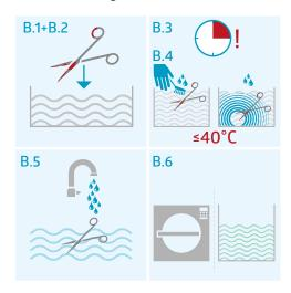
B.1 If deconex® INSTRUMENT PLUS has been used for pre-cleaning, use a second immersion bath for manual cleaning.
